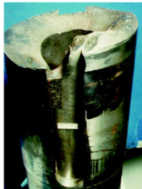
Left: Failure of an Output Shaft on an Emergency Backup Generator at a Powerplant due to Improper Hardness.
